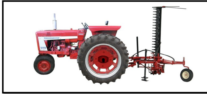
IH544 Tractor with a 2-Point Mounted Sickle Mower
